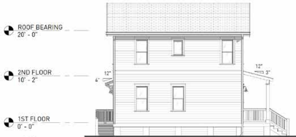
2 SIDE ELEVATION - 1 SD-3.1 1/8" = 1'-0"
